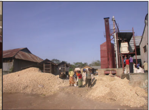
Recirculating dryer fuelled by shelled maize cobs.
